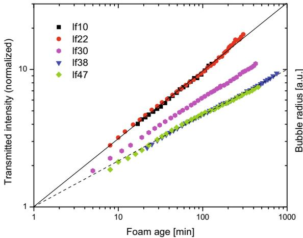
**Fig. 3.** The bubble size determined via the optical transmittance as a function of foam age is shown for five different liquid fractions. The plot is on doubly logarithmic scales indicating a power law dependence of the size with age. Straight lines with a slope of  $1/2$  (solid) and  $1/3$  (dashed) indicating the exponents of von Neumann and Ostwald dynamics are added for comparison.
