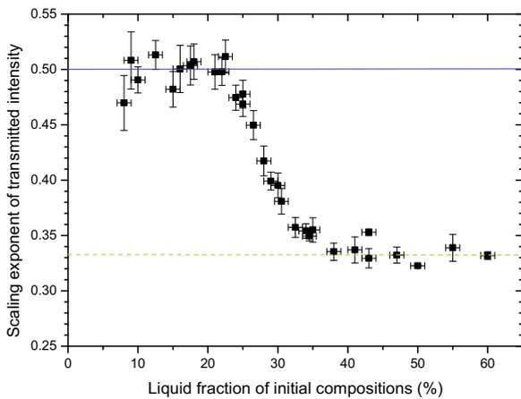
**Fig. 4.** The bubble growth exponent,  $\beta$ , determined from measurements as those shown in fig. 3 is shown as a function of liquid fraction (given in %). For comparison, the expectation of von Neumann dynamics,  $\beta = 1/2$ , and that of Ostwald ripening,  $\beta = 1/3$  is shown by the full and dashed lines, respectively. The transition between these two regimes is rather narrow at liquid fractions between 25% and 35%.
