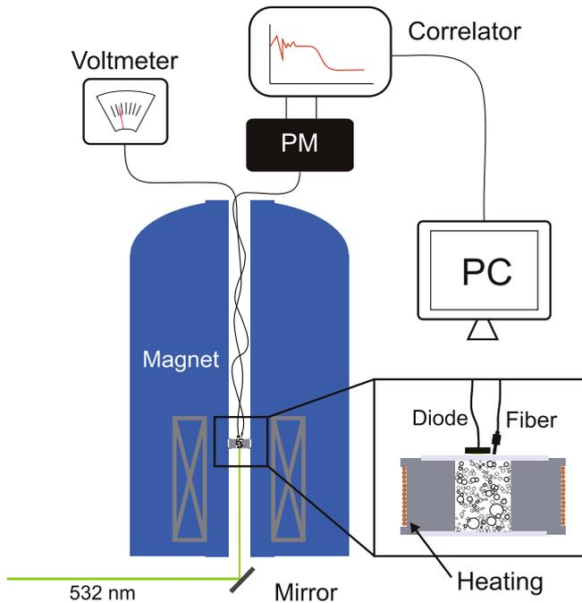
**Fig. 2.** Schematic illustration of the diamagnetic levitation setup. The foam sample cell, shown in detail in the inset, is illuminated from below and observed from above. The transmitted light is captured by a photodiode for the determination of the bubble size. A photomultiplier (PM) is used to determine the autocorrelation function to study the local dynamics.
