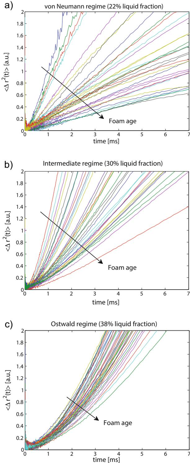
**Fig. 5.** The mean square displacement of scatterers in the foam is shown as a function of correlation time for three different liquid fractions (a: 22%, b: 30% and c: 38%). This shows the local dynamics of bubbles, which can be seen to be diffusive ( $\langle \Delta r^2 \rangle \propto t$ ) in the von Neumann regime and ballistic ( $\langle \Delta r^2 \rangle \propto t^2$ ) in the Ostwald regime.
